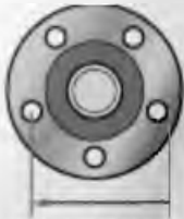
5-Lug Pattern Measure the distance from the center of one hole to the far side (not center) of a non-adjacent hole
